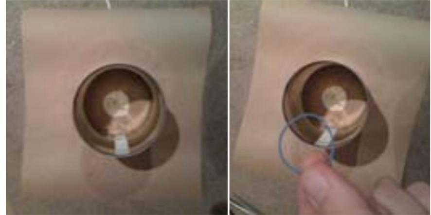
Now place the can on the paper so it is centered around your wooden disc. We will be folding the edges of our paper around the end of the can. I use a rubber band to help hold the paper in place while I wrap a piece of string around the end of the can.
